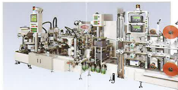
High-frequency Blood Bag Welding Machine
