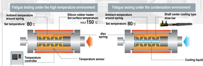
What effects occur on the disc springs when the inside of the main spindle of a machining center reaches a high temperature? What response measure should be taken in that case? To solve issues such as these, Tokaibane can implement fatigue testing with reproduction of the high temperature environment. We then make proposals that accurately describe those effects and their countermeasures
