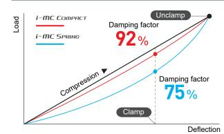
The i-MC COMPACT eliminates the load damping during compression that occurs with normal disc springs. This realizes an increase to the clamp load (decompression).
