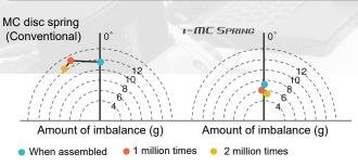
The i-MC COMPACT demonstrate excellent balanced performance on high performance machining centers that require ultra-high-speed rotation. The amount of imbalance is reduced to around 65% that of the conventional Tokai spring disc springs for machining centers (the MC disc springs). In addition, even after 2 million usages the balance characteristic of the spring remains mostly unaltered.
