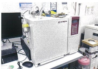
Analysis is performed using a gas chromatograph.
