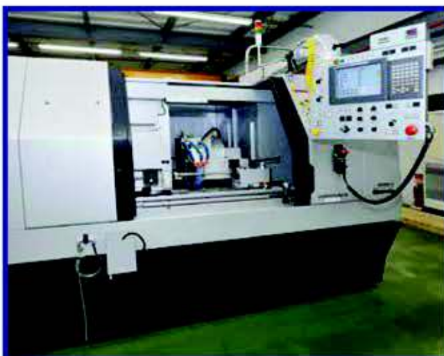
CNC Precision Cylindrical Grinder OGM250UNC III by Okamoto Machine Tool Works Co., Ltd. \phi 150 \times L500
