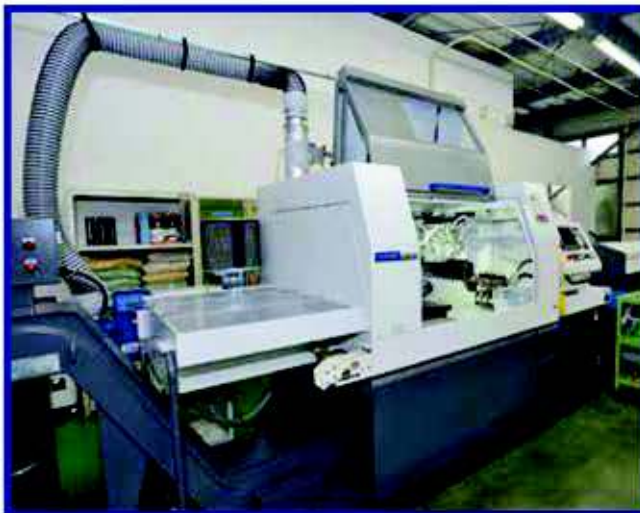
CNC Automatic Lathe L32X by Citizen Machinery Processing Diameters \phi 6 \sim \phi 32
