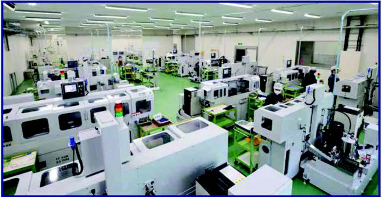
Small size and small-diameter gun drill processing area (20 units) – As of April 2018
