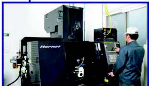
Ultra Precision Micro Fine Processing Unit Hornet by Roku Roku Sangyo Hole Diameters: \phi 0.05 \sim \phi 5.0 Revolution Frequency: 40,000rpm
