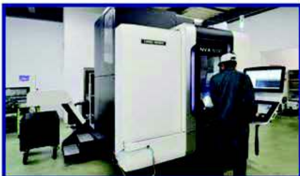
Solid machining center NVX5060/40 DMG by Mori Seiki Surface Dimensions: 600x400x300 Revolution Frequency: 15,000 rpm
