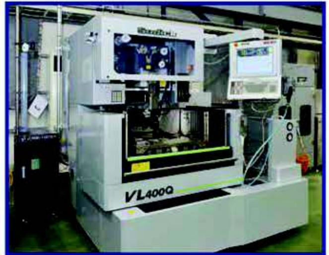
Wire Electric Discharge Processing Machine VL400Q by Sodick Table: 350 \times 250 \times 170
