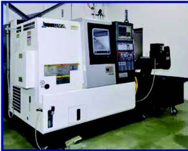
CNC Automatic Lathe LB2500EX II Okuma Processing Work: ~ \phi 150 \times L250
