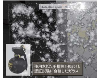
This is the glass passed the certification test, and a grenade that was used for the test.
